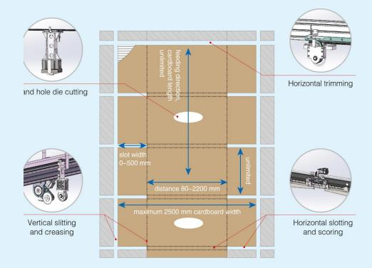
Board feeding, Slotting, Scoring, Slitting, Cutting, Trimming, Inline gluing option, All In One Compact Machine.
