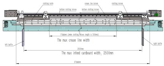
The width of the bottom slotting knives(totally together)
